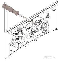
Fig. 56 Adjusting P2 CO<sub>2</sub> level
